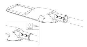
3. Loosen the screws to adjust the spigot and luminaire angle if necessary.
